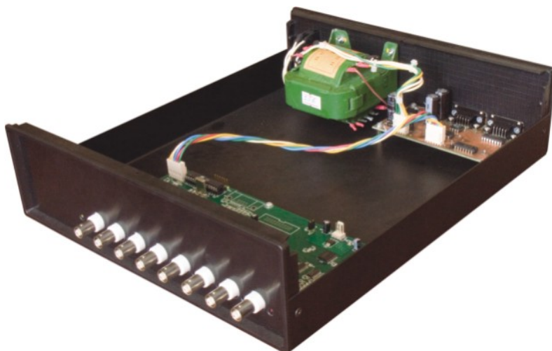
Figure 3 8 channel DAQ electronics for SEVAN detector.
